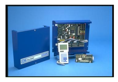
connection to achieve a completely stand-alone or networked full-function Building Automation System. The optional ManagePak<sup>TM</sup> Engineering Workstation host software for Windows<sup>TM</sup> running on PCs in a TCP/IP Server/Client based Ethernet provides more addresses, faster communication, and enhanced user interface features.
